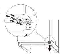
Remove the door fitting from the door bearing (1, 2). Move the bearing pivot from the right to the left hand hole (3). Place the door fitting supplied on the bearing pivot (4, 5).
